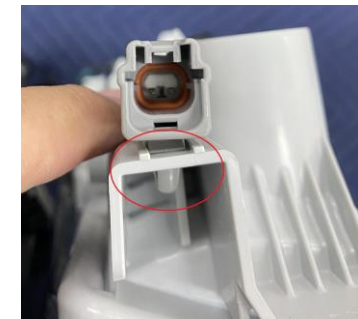
6. To remove the plug from car and take off clip from base of light.
