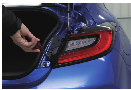
1. Open the trunk and unclip indicated hood. 2. To remove the 2 screws.
