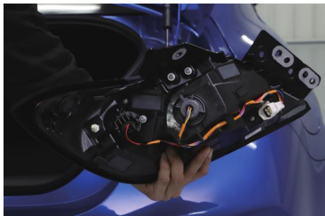
3. To remove the tail light and disconnect plug.
