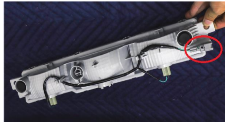
6. To remove the plug from car and take off clip from base of light.
