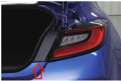
1. Open the trunk and unclip indicated hood. 2. To remove the 2 screws.
