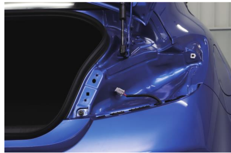
1. Open the trunk and unclip indicated hood. 2. To remove the 2 screws.
