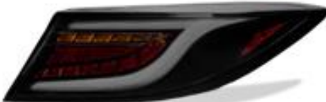
SBCAR(smoked lens.black base. white position. amber turning.red brake)
