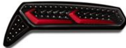
CBR(clear lens.black base.red position bar)
