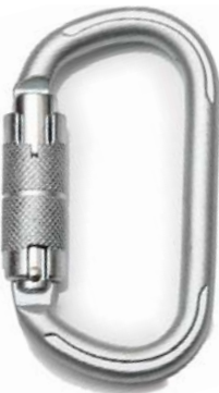
D Carabiner C2202 series Forged Alloy Steel Twist Lock Min. Breaking Strength: 23kN/5000lbs
