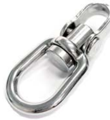
Swivel Combination I0202 series Alloy Steel Chrome Plated Min. Breaking Strength: 23kN/5000lbs
